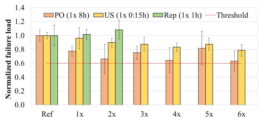
**Figure 4** – Normalized shear strength of RJS joints cyclicly aged [2].
